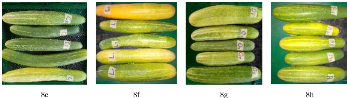
Figure 8: Stored cucumbers at initial and final stages of experiment: (a)Charcoal cooler bin (day one), (b) Laboratory (day one), (c) Open-Air (day one), (d) Refrigerator (Day one), (e) Charcoal cooler (day 14), (f) Laboratory storage (day 14) (g) Refrigerator (day 14), (h) Open-Air (day 14).
